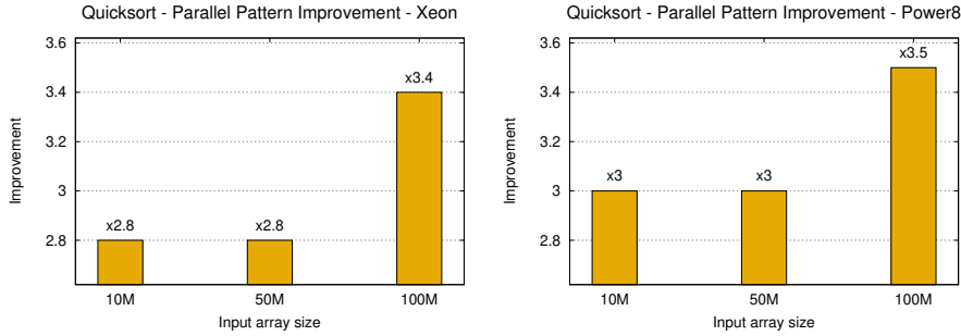
Fig. 7: Improvement of the PPs version compared to the “pure” AM version of the quicksort benchmark on the Xeon and Power8 platforms.
