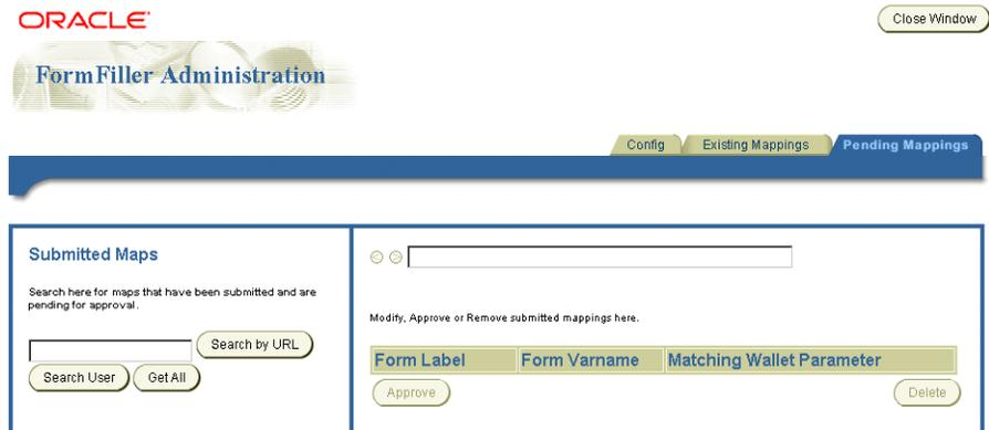
**Note:** For performance reasons, (such as a database connection cache with a five-minute expiration period) it can take up to five minutes for changes made using the Formfiller Administration to be reflected in the system.
