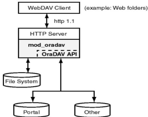
[Figure 7-1](#) shows a WebDAV client, such as Microsoft Web folders, passing HTTP requests to the Oracle HTTP Server. If the request is for content stored in the file system (not in an Oracle database), `mod_oradav` handles the access. If the request is for content stored in an Oracle database, the OraDAV API handles the access.
