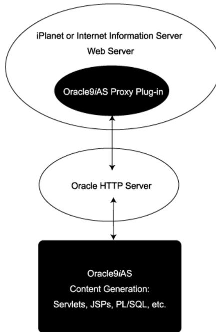
This proxy logic is provided as a plug-in, a shared library that is loaded by the third-party HTTP listeners. The plug-in uses APIs provided with the third-party listeners to directly handle HTTP requests, in much the same way that modules (mods) are plugged into the Oracle HTTP Server.
