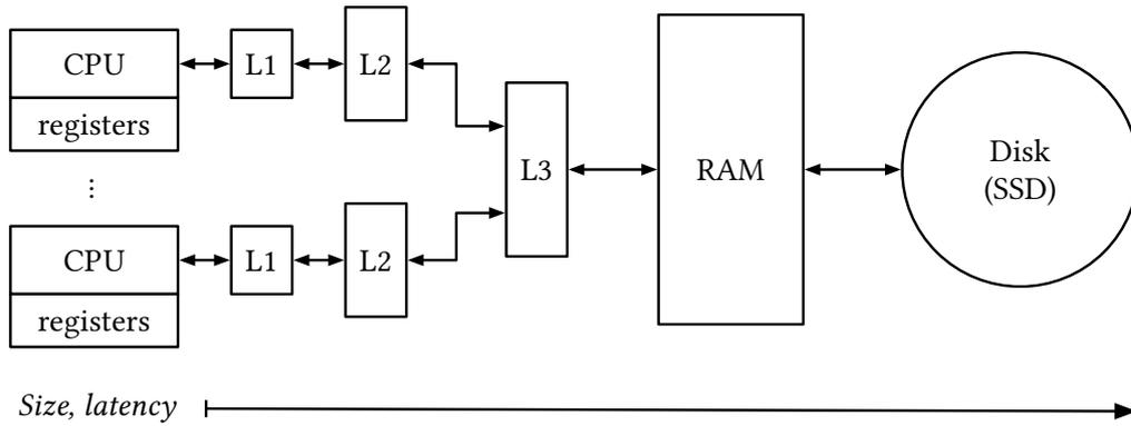
**Figure 1:** The computer memory hierarchy. From left to right, the memory size increases but latency increases as well.
