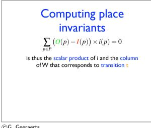
Computing place invariants  $\sum \left( O(p) - \mathbf{I}(p) \right) \times i(p) = 0$ is thus the scalar product of i and the column of W that corresponds to transition t Since this must hold for any t, we obtain: Theorem: any solution i to the following system of equations is a place-invariant:  $i \times W = 0$
