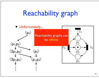
The reachability graph of a Petri net (aka the Transition System of a MultiSet Rewriting system) can be infinite
