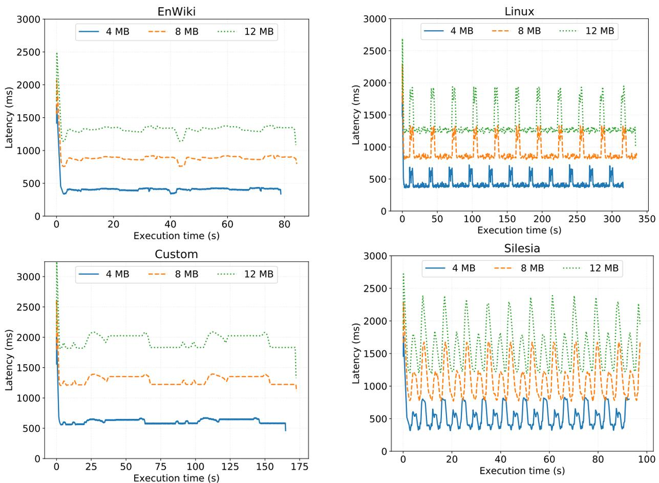
FIGURE 2 Latency variation over time with static micro-batch sizes.
