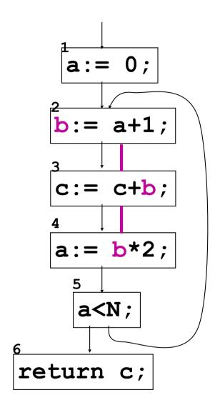
→ Two registers are enough: variables a and b will be never simultaneously live along the same arc
