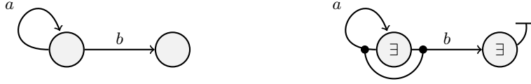
Figure 4: A possible query for graph simulation (on the left) and its translation in a guest for loose graph simulations (on the right).
