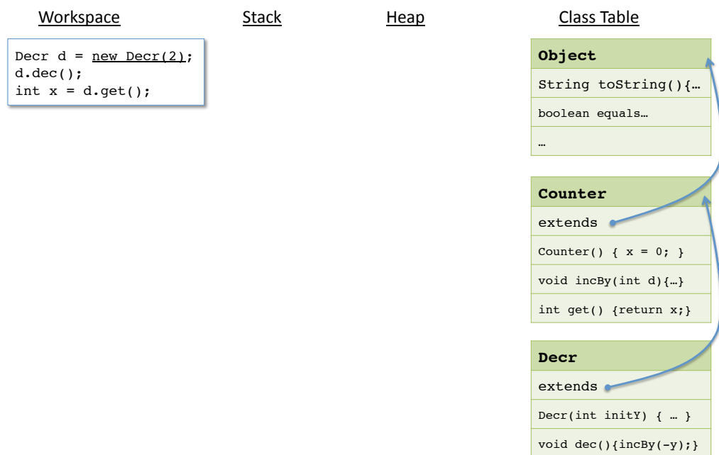
Figure 25.4: The initial state of the Java ASM example
