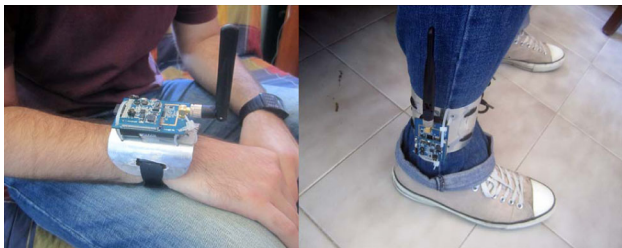
Fig. 3 Motes worn by the user are located on the right wrist, i.e., mote M_1 , and on the right ankle, i.e., mote M_2
