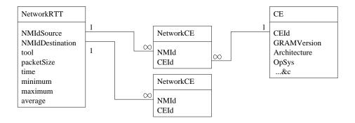
Figure 1: The linking between network monitor nodes and other grid edge nodes
